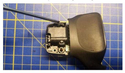
**Step 8.**Remove the 2 screws holding the pivot arm to the paddle shifter lever. Once removed, the pivot arm will
